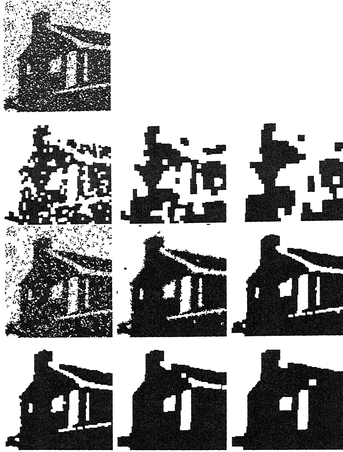
Figure 7 A noisy binary image (top row) and the output resulting from three different AS-filters (three subsequent rows), with increasing parameter n (from left to right). Refer to the text for further details.
